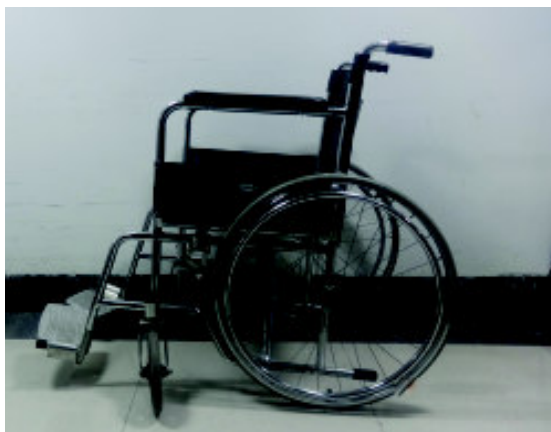
Figure 17.2 Conventional wheelchair, foldable frame, fixed arm rests, small castors
