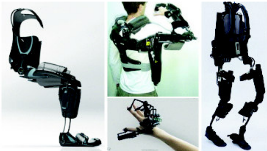
Fig 21.3 a) Erigo b) Hybrid Assistive Limb (HAL)
