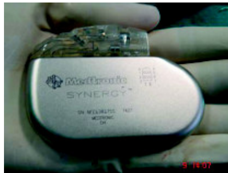
Figure 12: Neurostimulator that is connected to the electrodes and implanted in the upper chest wall below the skin
